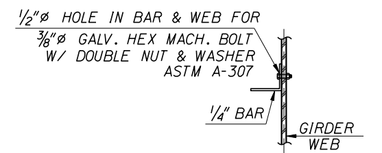
ALTERNATE CONNECTION DETAIL 1 1/2"=1'-0"
