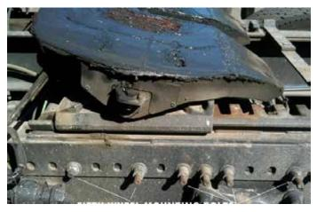
Figure 11.38 Fifth Wheel Mounting Bolts
