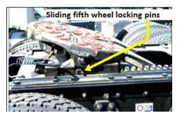
Figure 11.39 Sliding Fifth Wheel Locking Pins
