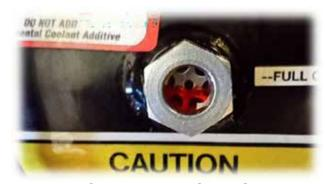
Figure 11.2 Coolant Level Sight Glass
