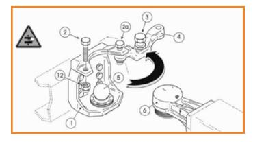
Figure 6.14 Drawbar Coupling Components
