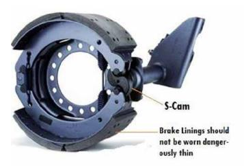
Figure 11.25 Brake Linings
