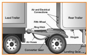
Figure 7.1 Converter gear on a dolly
