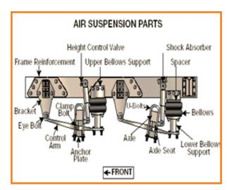
Figure 2.4 Air Suspension Parts
