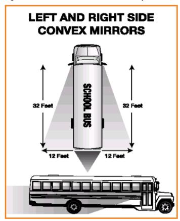
Figure 10.3 Left and Right Side Convex Mirrors
