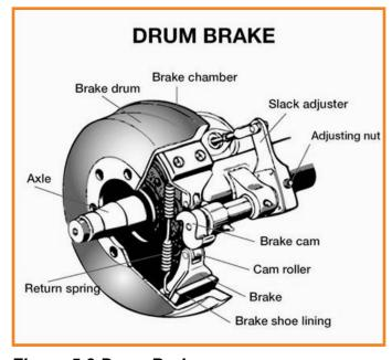
Figure 5.2 Drum Brake
