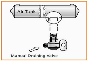
Figure 5.1 Air Tank Drain
