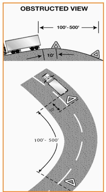
Figure 2.10 Obstructed View Triangle placement
