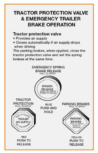
Figure 5.4 TPV and Brake Operation
