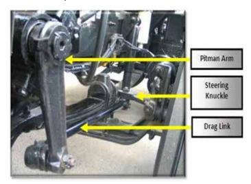
Figure 11.11 Steering Linkage
