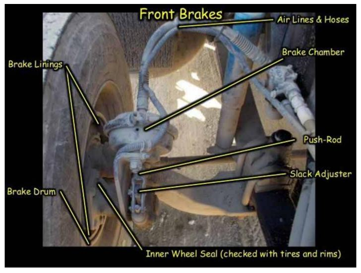
Figure 11.22 Front Brake Components
