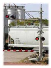
Figure 10.9 Gate / Flashing Red Light Signals
