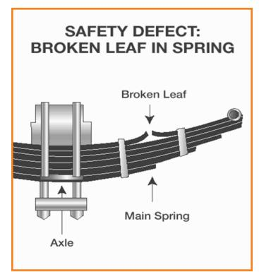
Figure 2.3 Broken Leaf Spring
