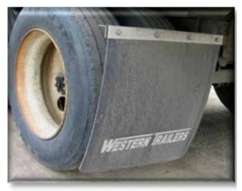
Figure 11.34 Properly Mounted Mud Flap
