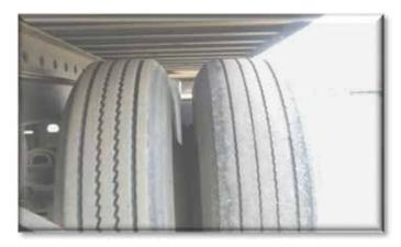
Figure 11.29 Proper Wheel Spacing
