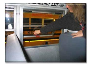
Figure 11.72 Window Alarm Check
