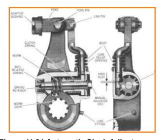
Figure 11.21 Automatic Slack Adjuster
