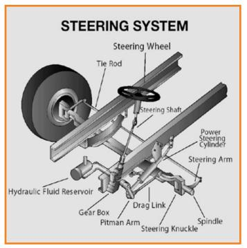
Figure 2.1 A typical steering system
