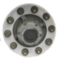
**Spacers or Budd Spacing:** An axle collar is placed between dual wheels to keep the wheels evenly separated.
