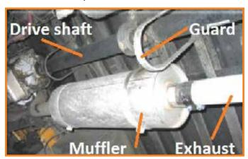
Figure 11.77 Under Bus Components
