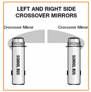
Figure 10.4 Left and Right Side Crossover Mirrors
