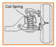
Figure 11.14 Coil Spring
