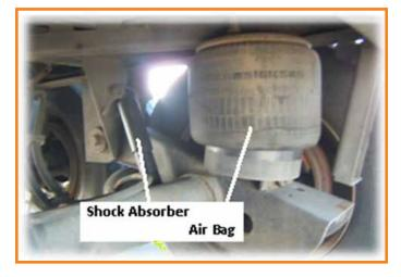
Figure 11.55 Shock Absorber and Air Bag
