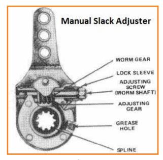
Figure 11.20 Manual Slack Adjuster
