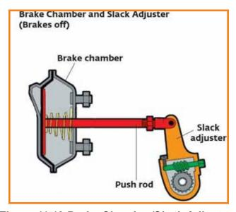
Figure 11.19 Brake Chamber/Slack Adjuster
