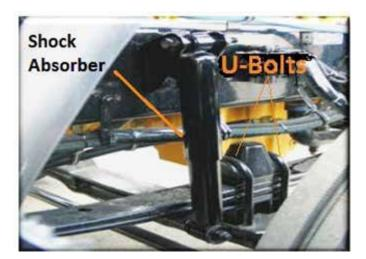
Figure 11.17 U-Bolts and Shock Absorber
