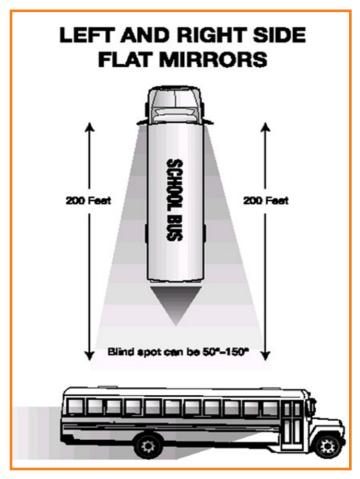
Figure 10.2 Left and Right Side Flat Mirrors
