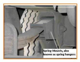
Figure 11.54 Spring Mounts / Spring Hangers
