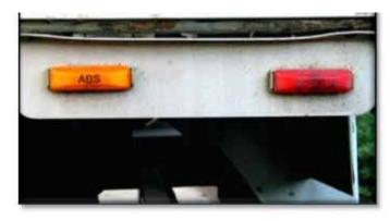
Figure 6.9 ABS Malfunction Warning Light
