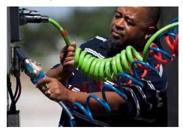
Figure 11.36 Secure Air and Electric Line Connections
