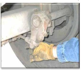
Figure 11.56 Slack Adjuster and Pushrod
