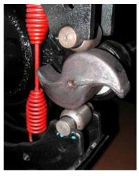
inside of the brake drum. When you release the brake pedal, the S-cam rotates back and a spring pulls the brake shoes away from the drum, letting the wheels roll freely again (**See Figure 5.2**).
