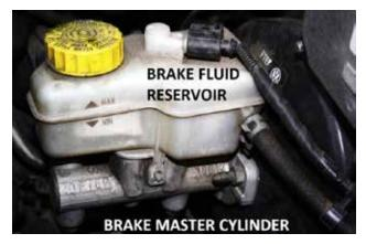
Figure 11.8 Master Cylinder and Brake Fluid
