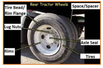
Figure 11.62 Rear Tractor Wheel Components
