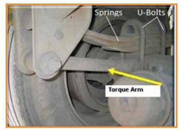
Figure 11.53 Torque Arm, U-Bolts, and Springs
