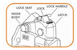
Figure 6.11 Lock Components
