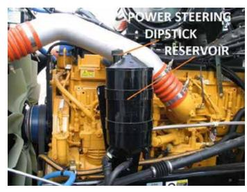
Figure 11.4 Power Steering Components
