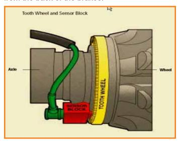
Figure 2.19 Tooth Wheel and Sensor Block
