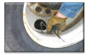
Figure 11.59 Checking Tire Pressure
