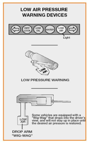
Figure 5.7 Low Air Pressure Warning
