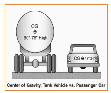
Figure 8.1 Center of Gravity
