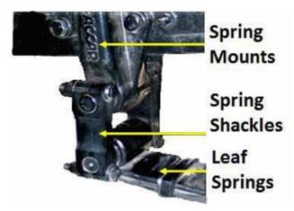
Figure 11.12 Leaf Spring Suspension Components
