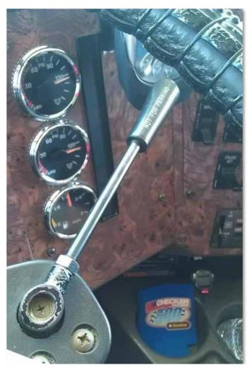
The trailer hand valve on this International tractor is located on the steering column. Figure 6.7 Trailer Hand Valve
