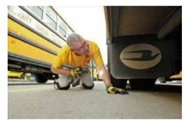
Figure 11.79 Under Bus Frame Check
