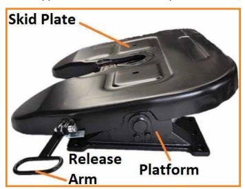
Figure 11.42 Fifth Wheel Skid Plate Components
