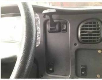
Trailer Brake Handle in Freightliner Tractor
