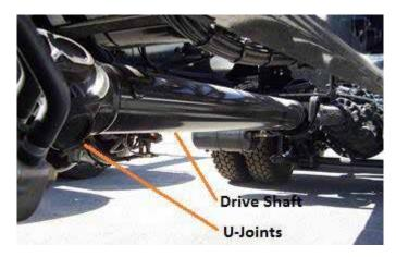
Figure 11.31 Drive Shaft and U-Joints
