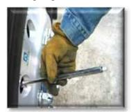
Figure 11.28 Checking Proper Tire Inflation
