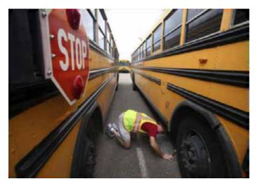
Figure 11.76 Under Bus Fuel Leak Check
