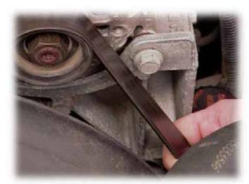
Figure 11.3 Checking Belt Tension
