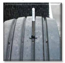
Figure 11.28 Checking Tire Tread Depth
