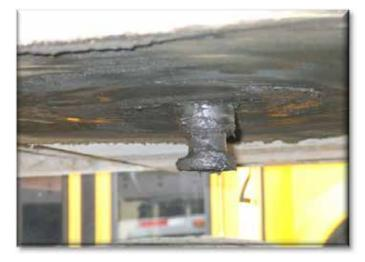
Figure 11.44 Trailer Kingpin and Kingpin Plate
