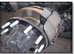
Figure 11.57 Brake Drum and Brake Rotor
