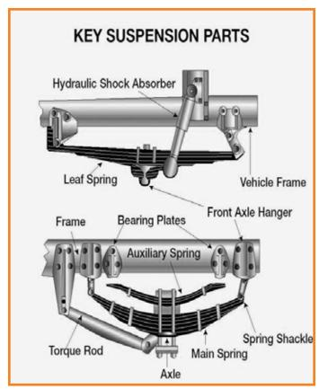
Figure 2.2 Key Suspension Parts
