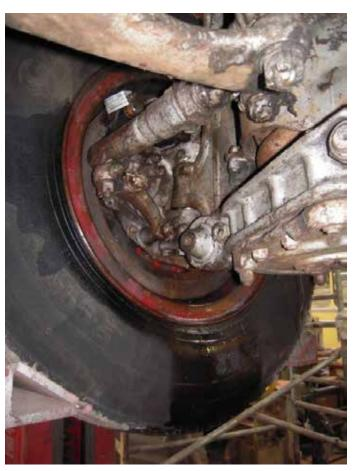
Figure 11.26 Brake Mounts
