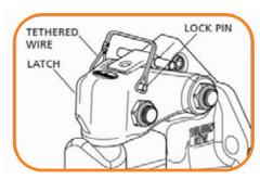
Figure 6.10 Lock Pin and Latch
