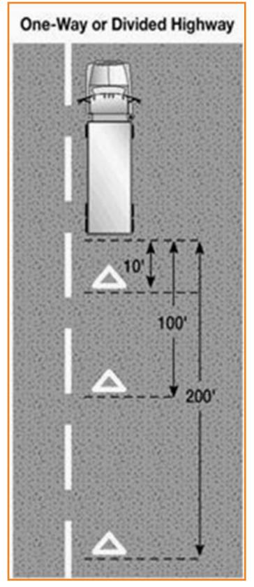
Figure 2.8 Placing Warning Devices
