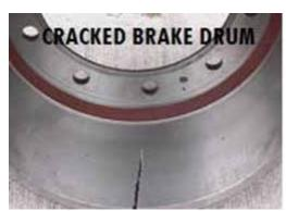
Figure 11.24 Cracked Brake Drum
