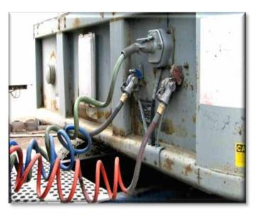
Figure 11.49 Trailer Air and Electrical Connections
