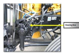
**Steering Linkage:** Transmits steering action from steering box to front wheels
