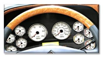
**Oil Pressure Gauge**: As soon as the vehicle is started, check the oil pressure gauge to make sure the engine has oil pressure. Too little pressure can ruin the engine.
