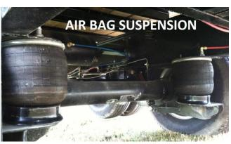
**Spring Mounts:** Consist of the brackets, bolts, shackles, and bushings used for attaching springs and/or air bags to vehicle frame. Loose, worn, or broken components may lead to loss of vehicle control or rollover.
