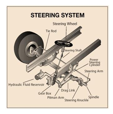
Figure 2.1 illustrates a typical steering system
