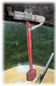
automatic wig wag will rise out of your when view the pressure the in system goes above 55 psi. The manual reset type must be placed in the "out of view" position manually, and it will not stay in place until the pressure in the system is above 55 psi.
