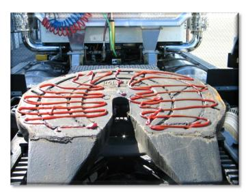
☐ Be sure that the fifth wheel plate is greased as required. Failure to keep the fifth wheel plate lubricated could cause steering problems because of friction between the tractor and trailer.
