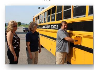
Check to see that fuel access door (if equipped) is securely latched.
