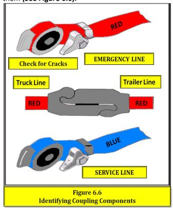
**Figure 6.6 Coupling Components**
