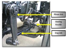
Check for loose or missing nuts, bolts, or cotter pins.
