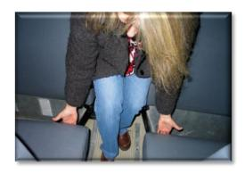
Check to see that seats are firmly attached to the floor.
