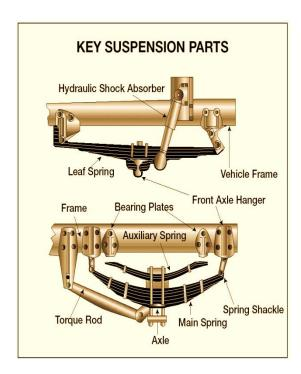
**Figure 2.2 Key Suspension Parts**
