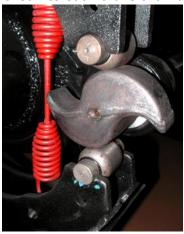
the rod out, moving the slack adjuster, thus twisting brake camshaft. This turns the S-cam (so called because it is shaped like the letter "S"). The S-cam forces the brake shoes away from one another and presses them against the
