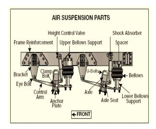
Figure 2.4 Air Suspension Parts
