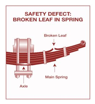
Figure 2.3 Broken Leaf Spring
