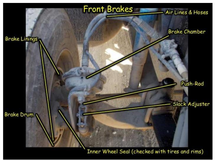
**Brake Drum or Rotor:** Brake linings, or pads, rub on the inside of the drum or on the rotor to slow the vehicle down.
