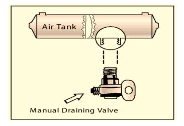
Figure 5.1 Air Tank Drain
