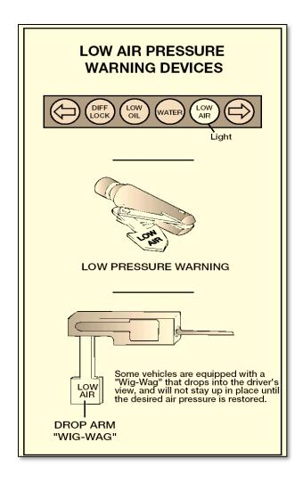
Figure 5.5 Low Air Pressure Warning
