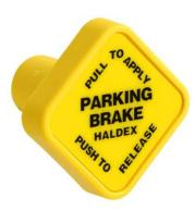
out to apply the parking brakes, push it in to release. The control will be diamondvellow. shaped knob labeled "parking brake" on newer vehicles. On older vehicles, it may be a round blue knob
