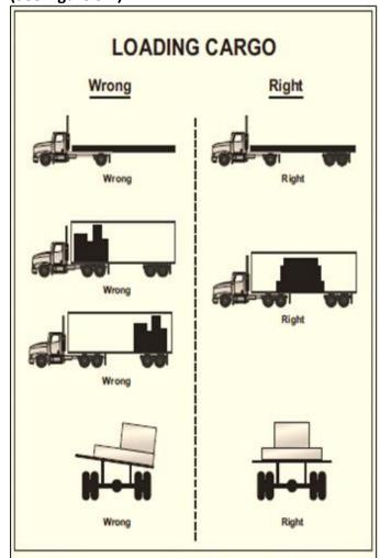
Figure 3.1 Loading Cargo Correctly
