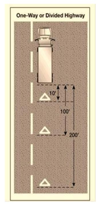
Figure 2.8 Placing Warning Devices
