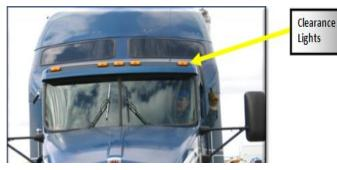
Clearance and rear identification lights mark the "overall width" of the design dimension of the widest part of the vehicle, exclusive of the signal lamps, marker lamps, outside rearview mirrors, flexible fender extension and mud flaps. Clearance and identification lamps are required on most buses, trucks and trailers that are 80 inches or more in overall width. Red light on rear corners of vehicle and/or trailer(s).
