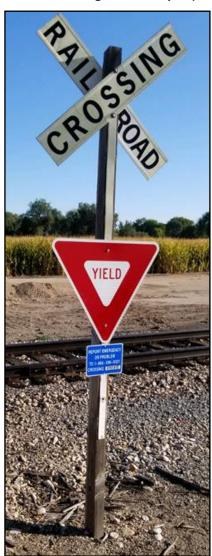
defined as "passive" - crossings that do not have "active" features such as flashing red lights or crossing gates that block the approach to railroad tracks.
