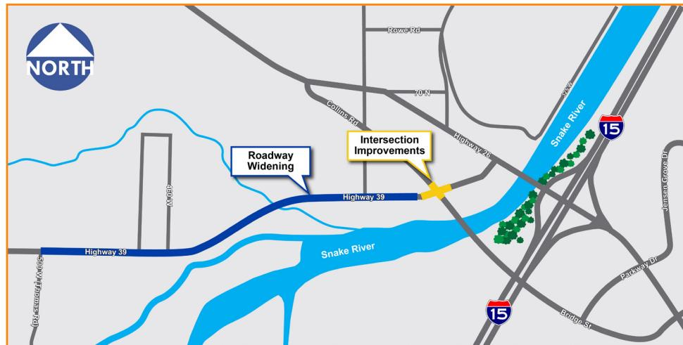
**What improvements are being designed?** SH 39 from approximately Thomas Road to Collins Siding Road will be widened with a continuous center turn lane to provide safety improvements for increasing traffic volumes in the corridor. When ITD designed this section of SH 39 decades ago, they planned for a future widening by purchasing adequate right-of-way. This will allow the project to proceed with very little, if any, impacts to private property.
