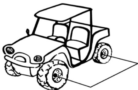
**Wheelbase** is the distance between the center of the front axle and the center of the farthest rear axle
