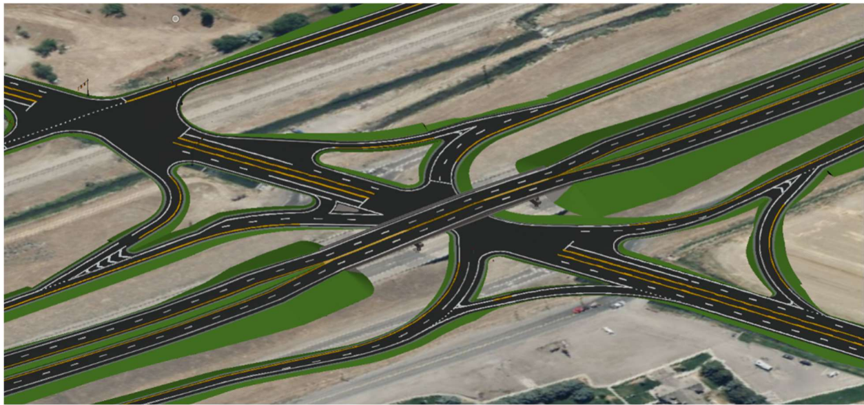
Figure 26: SPUI at County Line Road
