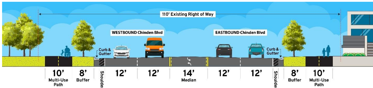
Figure 14. Glenwood St. to Kent Ln. Cross Section
