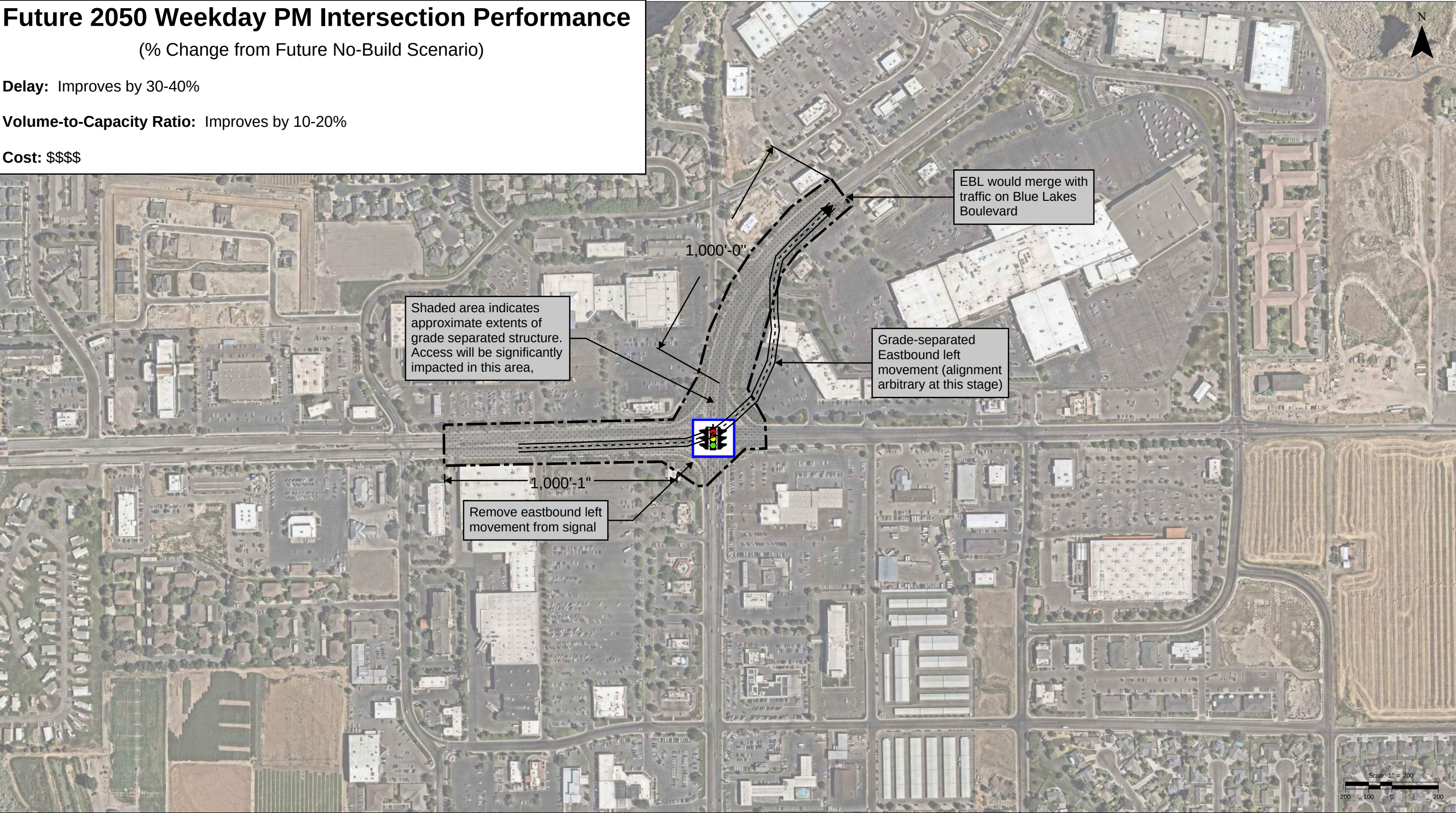
Initial Alternatives Eastbound Left-Turn Flyover Ramp Twin Falls, Idaho Figure GR2
