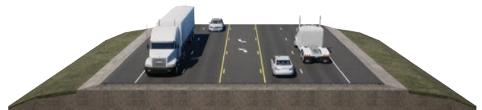
Four-Lane Highway with Center Turn Lane
