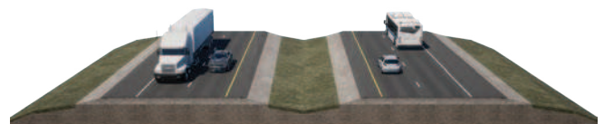
Four-Lane Divided Highway
