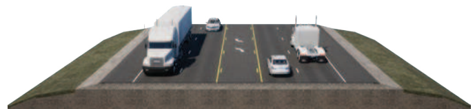
Four-Lane Highway with Center Turn Lane
