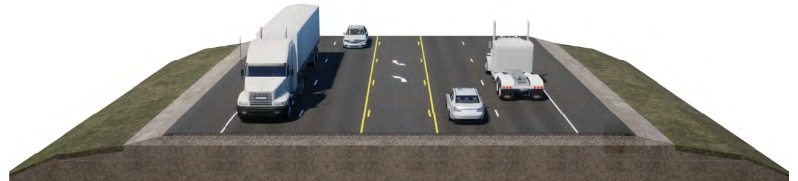
Four-Lane Highway with Center Turn Lane
