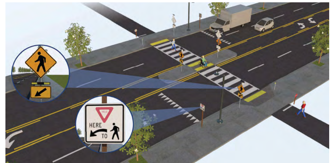
Examples of a bike lane and crosswalk
